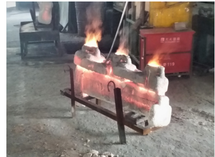
Above: Installation of handrail on site. down: Fabrication of the cast stainless steel posts.
