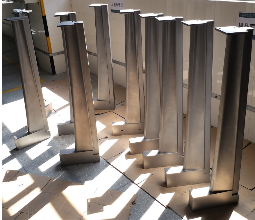
Above: Installation of handrail on site. down: Fabrication of the cast stainless steel posts.
